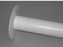
Using a fin as a guide, position the remaining undrilled centering ring onto the motor tube as shown. Mark the position of this centering ring. DO NOT GLUE THE FIN IN AT THIS TIME. Remove the fin and slide the centering ring back toward the aft centering ring.
