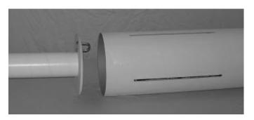
Epoxy the lower body tube support ring (10" diameter coupler section 3 15/16" long) into the aft end of the lower body tube. The lower body tube support should seat against the lower centering ring and also be flush with the end of the body tube. This ring adds support to the lower body tube to prevent damage from landing.
