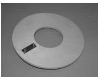
Epoxy the forward centering to the motor tube. Apply a fillet of epoxy around the motor tube as shown.
