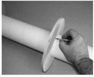
The fin is slid back so that when epoxy is applied to the motor tube to hold the ring, there will be no bead of epoxy where the fin will rest (between these two rings). Apply a bead of epoxy aroung the motor tube where this ring will rest and slide it back into position.
