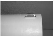
Epoxy the nose cone bulkhead into the nosecone. Use plenty of epoxy here and take care not to push the nose cone bulkhead too hard into the nose cone, it will deform the nose cone. Apply a fillet of epoxy around the joint, stand the nose cone up point downward and allow to cure completely.
