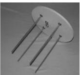
Install the U-Bolt in the lower electronics bay bulkhead with the U-bolt on the opposite side of the machined lip.
